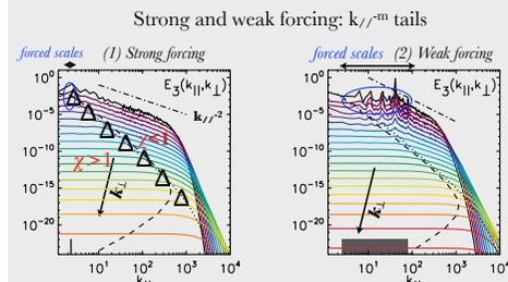
• Energy in  $\chi < 1$  region:  $E_3(k_{\perp}, k_{\parallel}) \propto k_{\parallel}^{-2} r^m$  due to  $1/f^{\circ}$  spectrum of large  $\perp$  eddies
