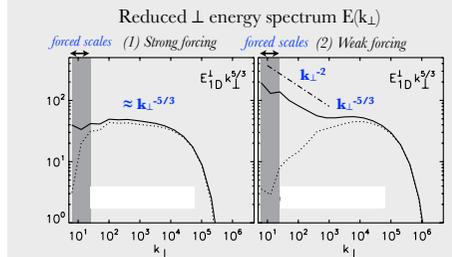
Dotted: reduced spectra obtained from 3D spectra after suppressing excitation in region  $\chi < 1/2 \Rightarrow$  suppresses  $k_{\perp}^{-2}$  weak scaling (right)
